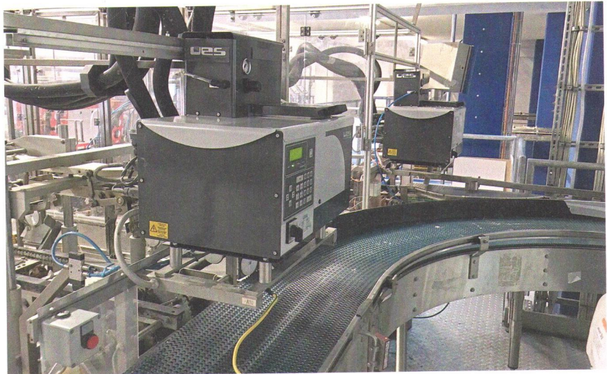
Hot glue equipment integrated into the packaging process enables a long shelf life for cardboard packaging.
